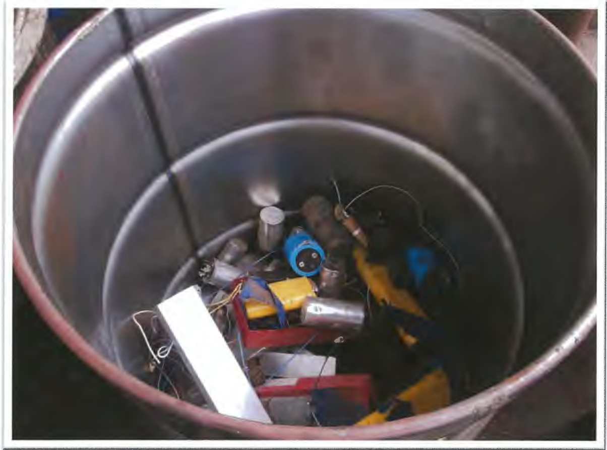
Photo 2: Accumulated PCB waste
