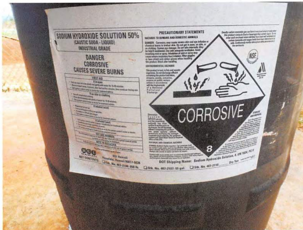
Sodium Hydroxide solution used to clean microfiltration units (performed quarterly).
