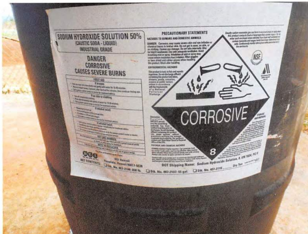
Sodium Hydroxide solution used to clean microfiltration units (performed quarterly).
