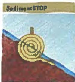
SedimentSTOP is more porous than a wattle, allowing it to perform as a buffer strip that slows water and filters sediment. In the event that water does flow over the top, SedimentSTOP has an attached Splash Apron, which reduces rill formation and potential down slope erosion.
