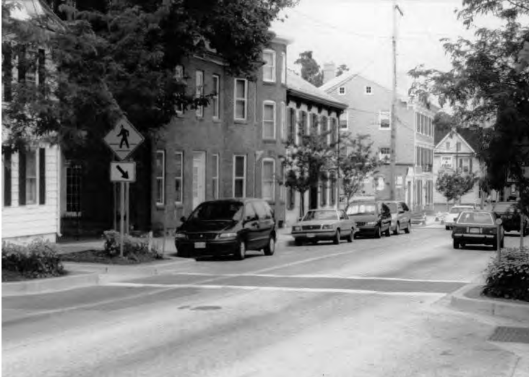
Figure 34. Curb Extension at a Mid-Block Crossing (Choker) with Textured Crosswalk and Landscaping – Westminster, Maryland (24).
