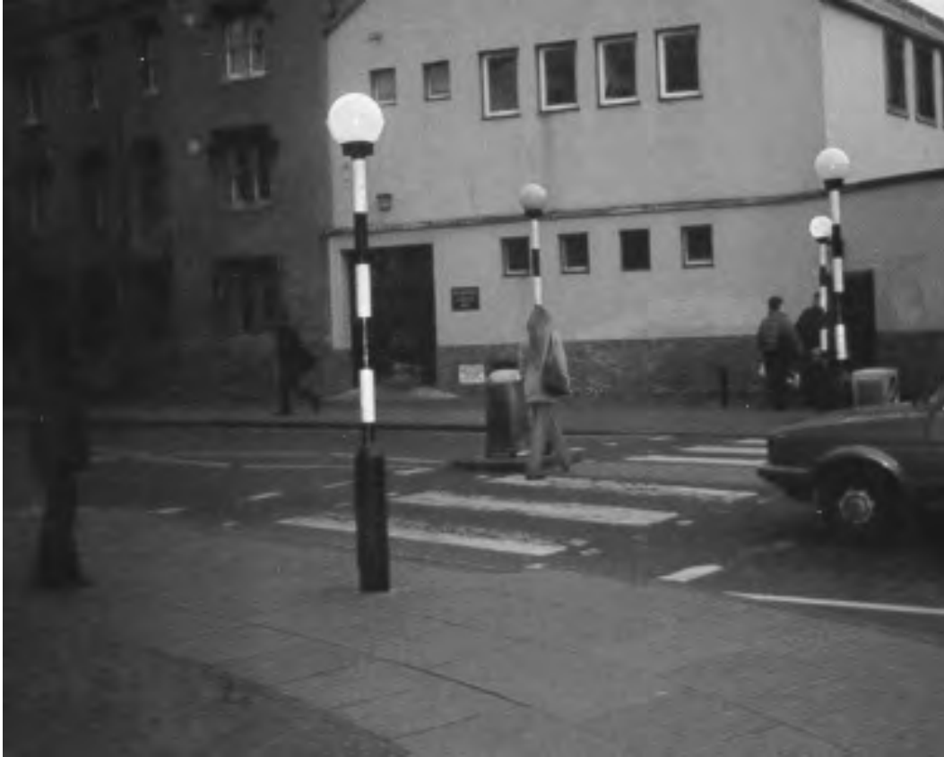
Figure 30. Use of Belisha Beacons at Zebra Pedestrian Crossings – United Kingdom. (Photo courtesy of Herman Huang, UNC Highway Safety Research Center)
