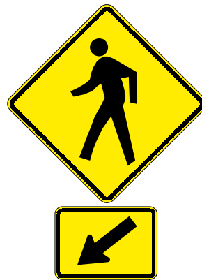
Figure 14. Pedestrian Crossing Sign (W11-2) with Supplemental Plaque (W16-7) (11).
