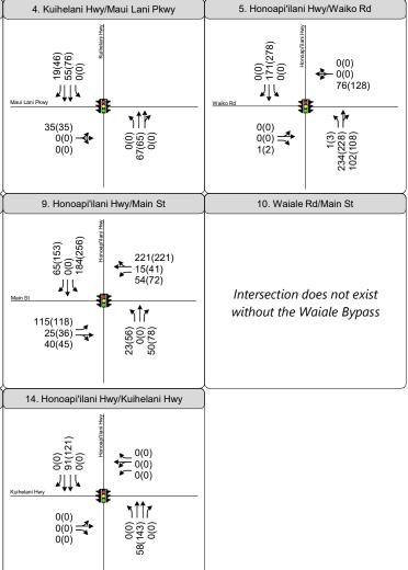
Figure 3 Peak Hour Traffic Volumes and Lane Configurations Net New Project Only, Phase 1 (2022)
