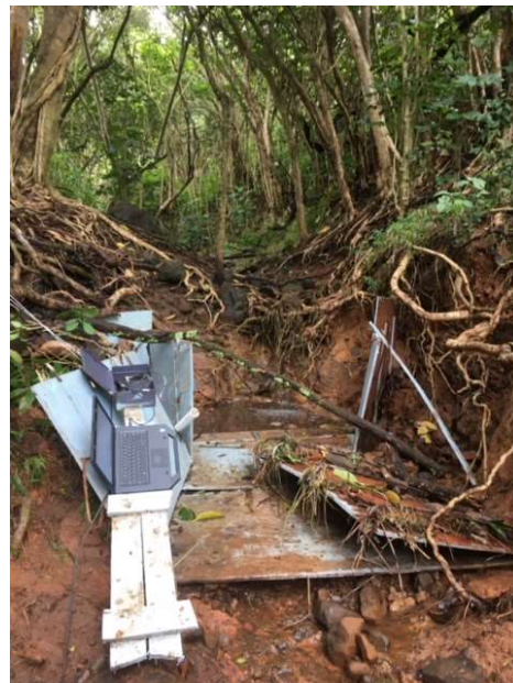
2/18/18 Storm Hydrograph and Resultant Damage to Lipalu Flume Where the Depth of Water Exceeded 4.5 Feet
