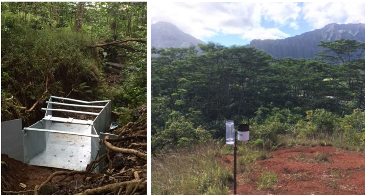
Wooden 108-inch length, 48-inch wide cutthroat flume and rain gauges installed within watershed
