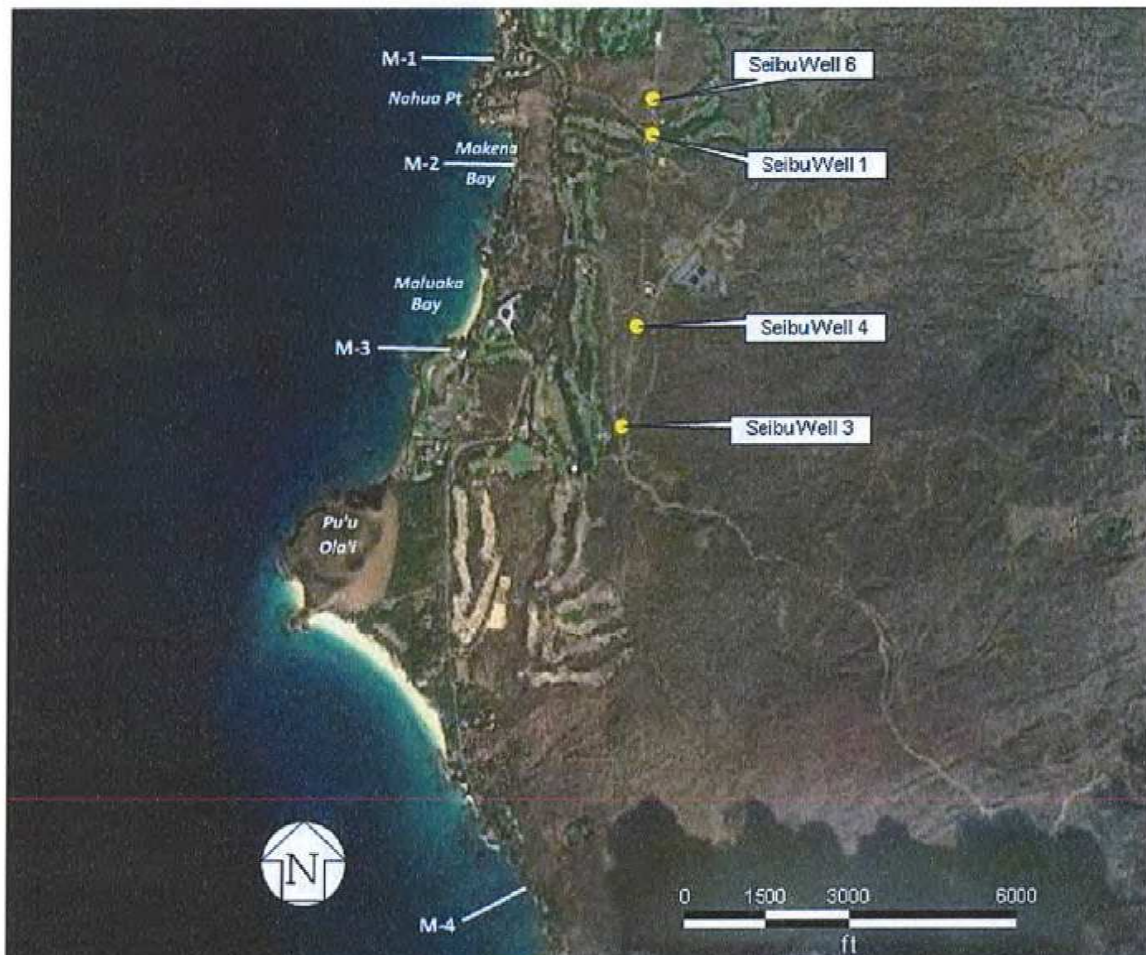
Figure 1. Location of quarterly water quality transects (M-1 through M-4) and irrigation wells.
