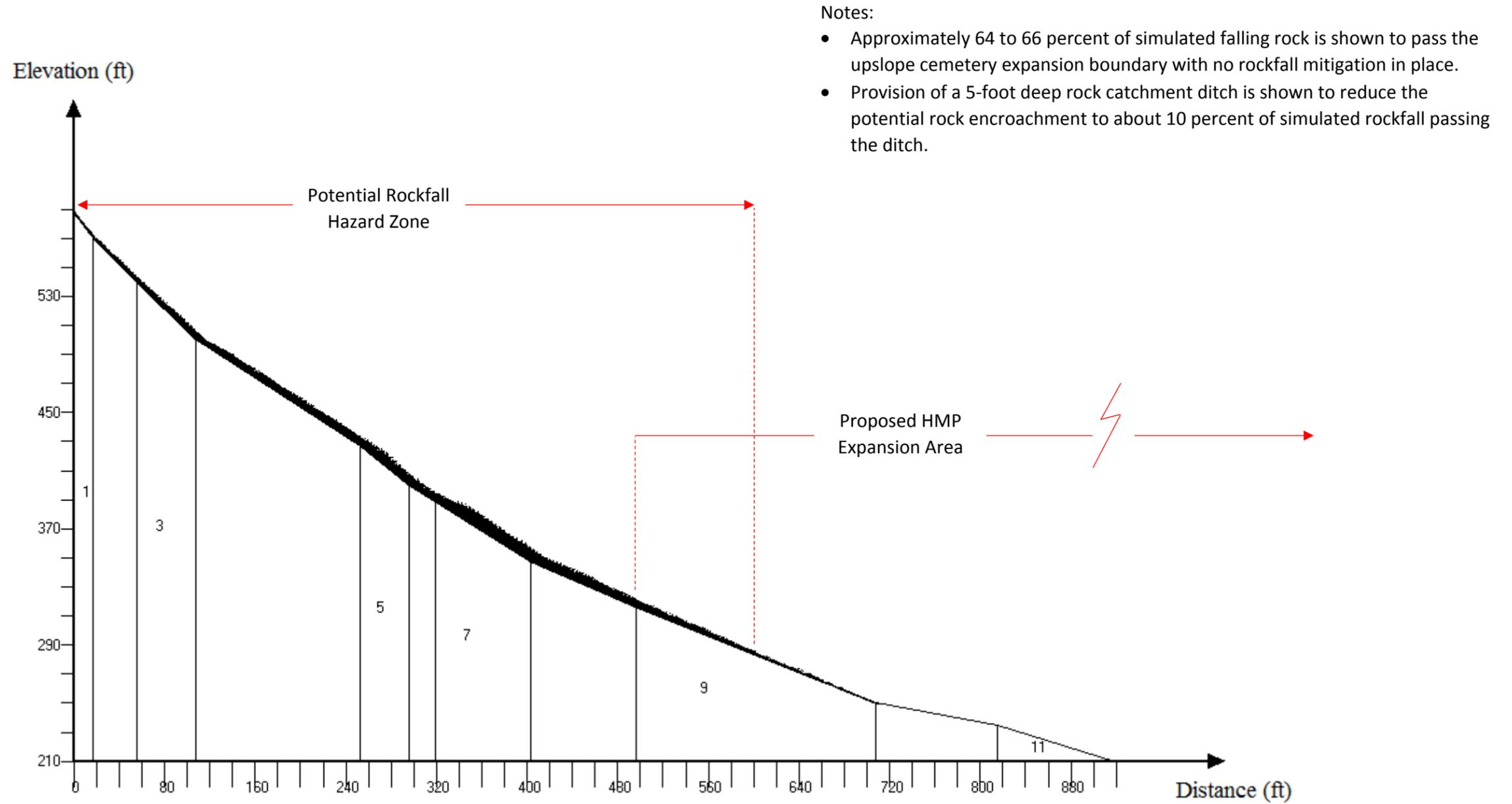
**POTENTIAL ROCKFALL SIMULATION – SLOPE PROFILE “A”**
