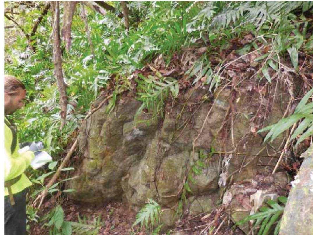
Photograph No. 43: (2587) Fractured and highly weathered rock outcropping at the eastern portion of the PRSA-2 area shown on the Site Plan, Plate 2. (Wpt. OC11).
