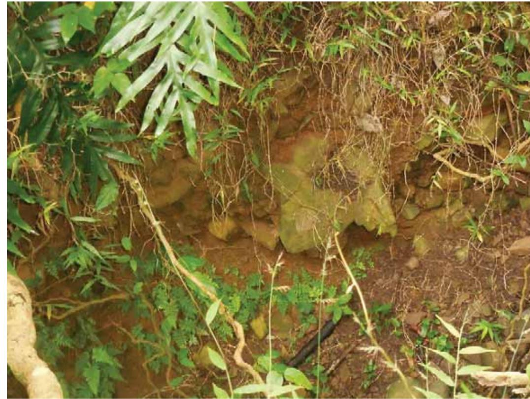
Photograph No. 51: (2612) Existing scoured shallow subsurface exposure showing conditions that appear to represent older alluvial/colluvial soil deposits containing appreciable rock fragments consisting of gravel, cobbles, and boulders. The location is within the lower central basin area. (Wpt. 0161)
