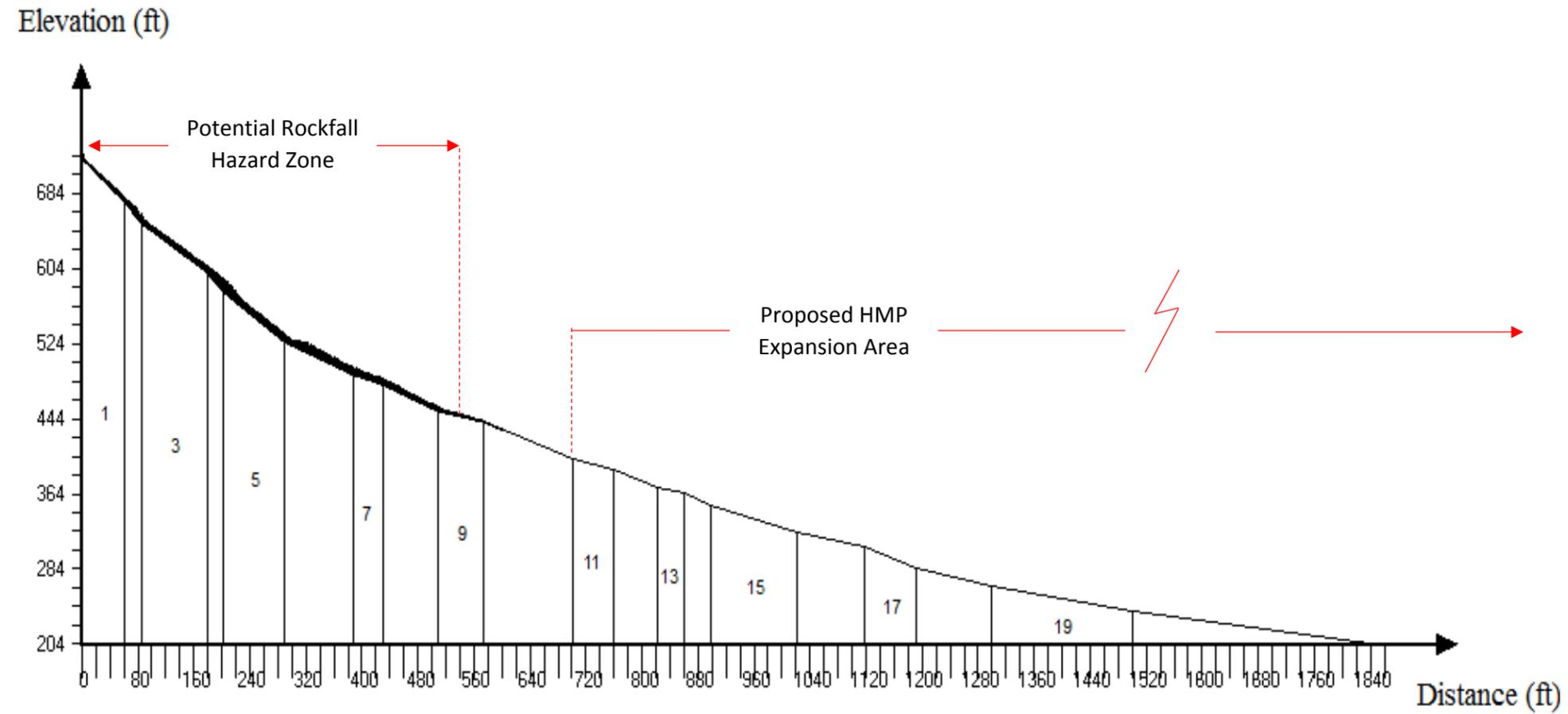
**POTENTIAL ROCKFALL SIMULATION – SLOPE PROFILE “C”**
