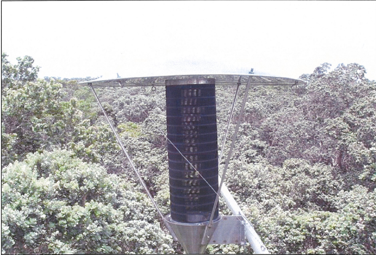
Figure 6. Standard open-site fog gauge with collection screen (black) and rain shield “hat”.
