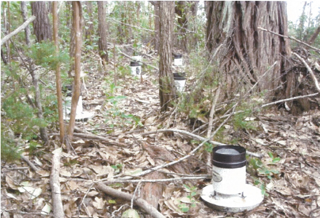
Figure 10. Multiple rain gauge (n = 15) throughfall sampling under Eucalyptus
