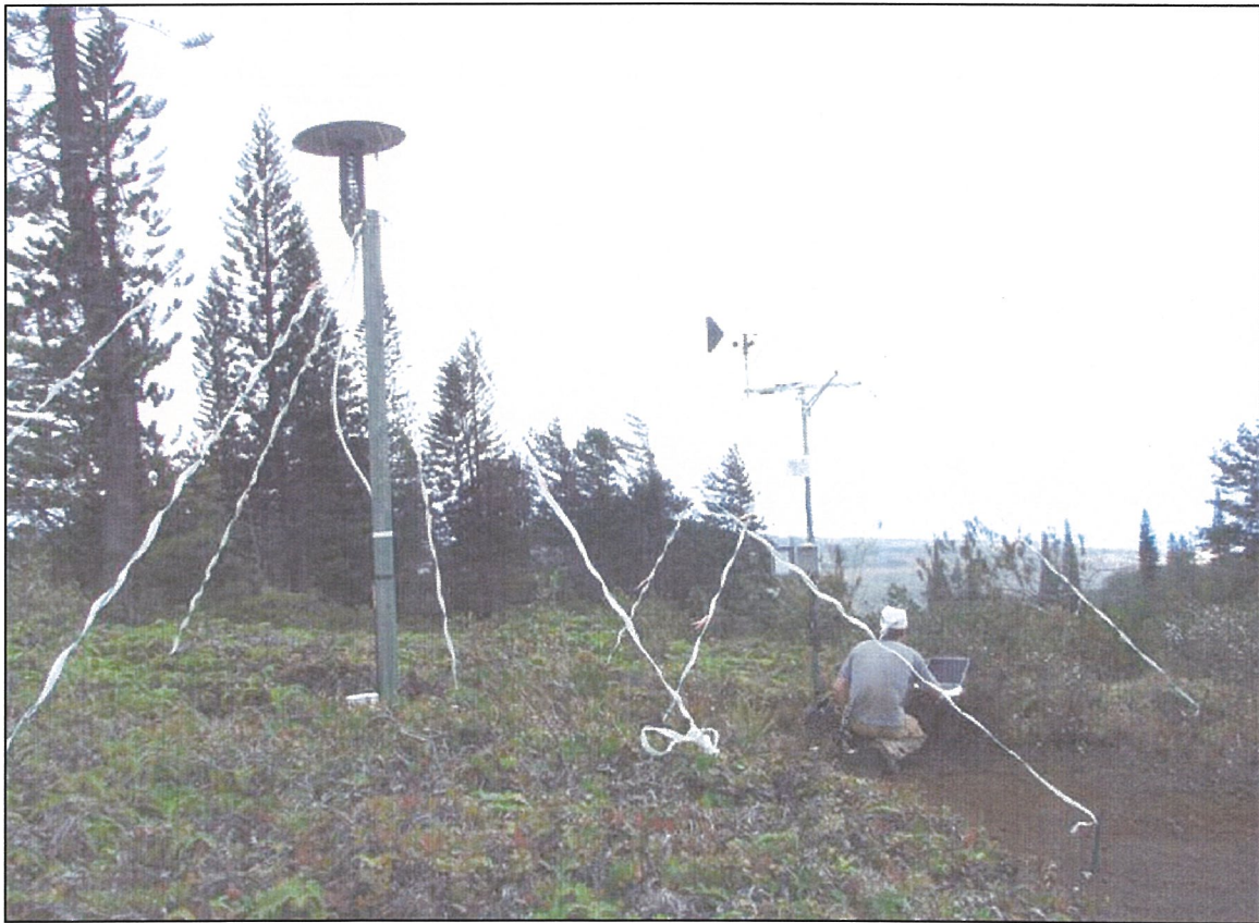
Figure 5. Open-site meteorological station, fog gauge at left.
