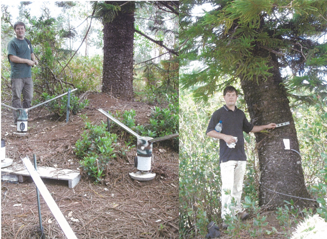
Figure 8. Throughfall collectors under Cook pine, including “trough-gauges” and standard rain gauge (center extreme left). Stem-flow collector visible on tree at right.
