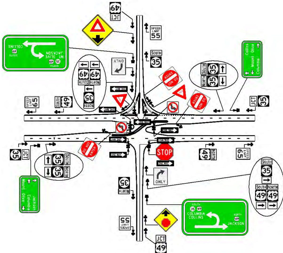
Figure 23 – Recommended J-Turn Intersection Signing Treatment
