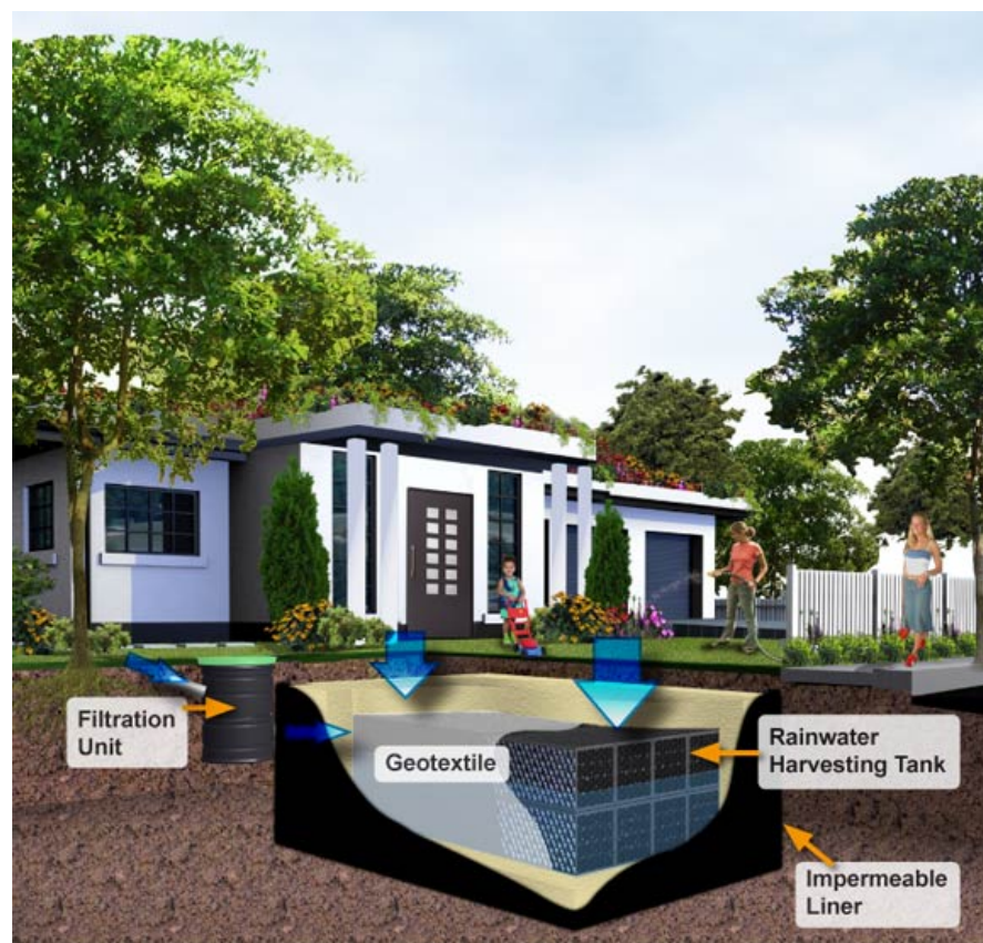
Figure 2-6. Schematic of a subsurface tank
