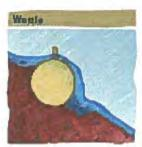
Wattles create a dam-like structure that causes water to back up and flow over the top, resulting in potentially severe erosion on the down slope side of the wettle.
